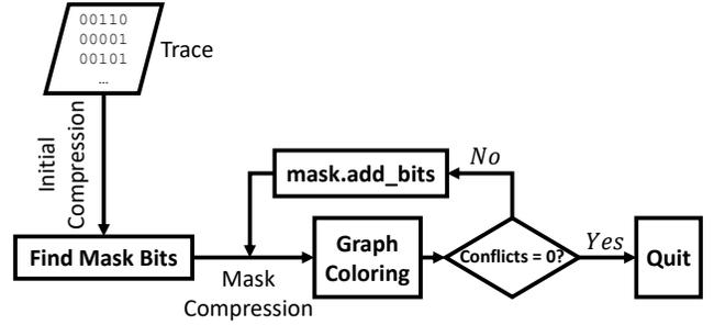
Figure 4: General structure of the proposed flow.
