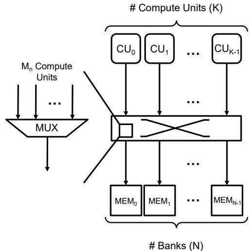
Figure 1: Hardware template for memory banking.
