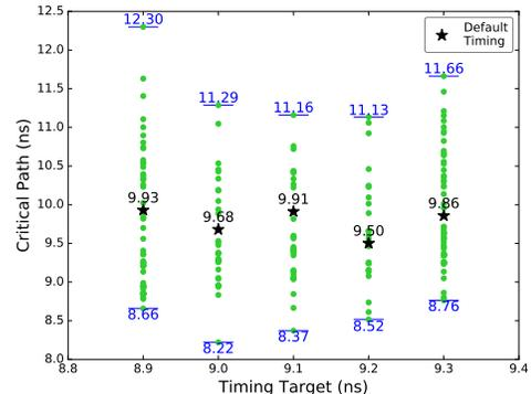
Fig. 1. Timing distribution of `bfly` for various tool settings and timing constraints – x-axis represents target clock period (ns), and y-axis represents critical path delay (ns).
