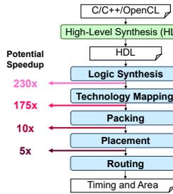
Fig. 2. Potential speedups by leveraging QoR inference at different stages
