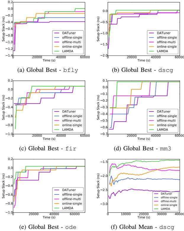
Fig. 4. Timing closure of *bfly*, *dscg*, *fir*, *mm3*, and *ode* using DATuner, *offline-single*, *offline-multi*, *online-single*, and LAMDA – (a)-(e) Best timing results achieved over time. (f) Mean of all timing results visited over time.
