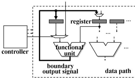
Figure 1: Generic structure of the FSM model.
