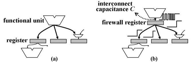
Figure 2: The insertion of a firewall register.
