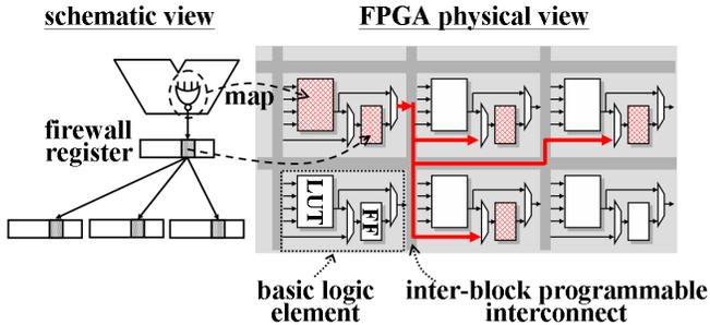
Figure 3: Firewall register implemented in a modern FPGA.
