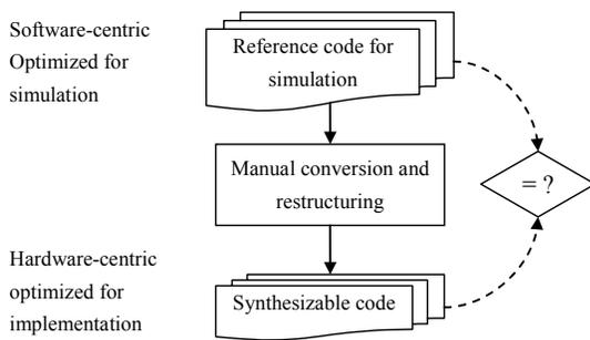
**Figure 1: Manual code modification for hardware synthesis.**
