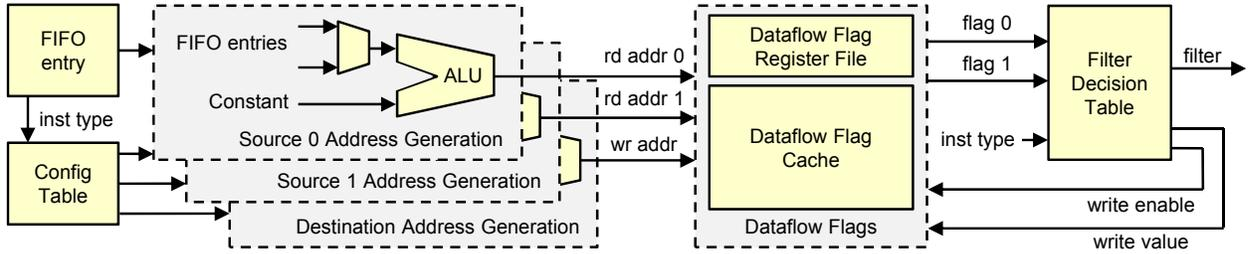
Fig. 5: Hardware architecture of the dataflow engine.
