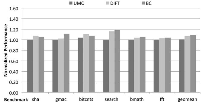
Fig. 6. The performance overheads of run-time monitoring on the Harmoni co-processor. The Y-axis shows normalized performance relative to an unmodified Leon3 processor. The X-axis shows the names of benchmarks used in the evaluation.
