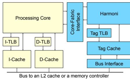
Fig. 3. High-level block diagram of the Harmoni architecture.
