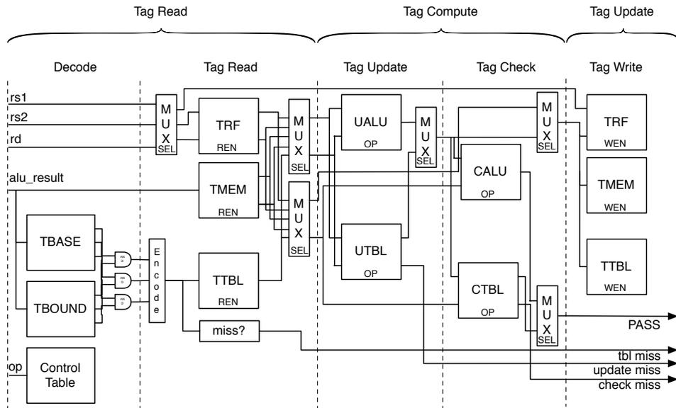
Fig. 4. High level block diagram of the Harmoni pipeline. The pipeline can be broken down into five discrete stages. The first two stages read the tags of operands used in the instruction, the third and fourth stage update and check the tags, the fifth stage writes the updated tag. The output of the control table is connected to all of the modules in the last four stages of the pipeline and determines their behavior.
