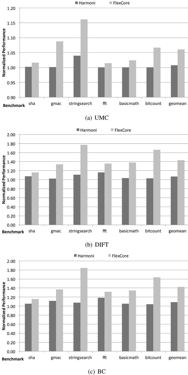
Fig. 7. Normalized performance overheads of run-time monitoring on the Harmoni co-processor and the FPGA-based co-processor (FlexCore) for a main processing core running at 1GHz.
