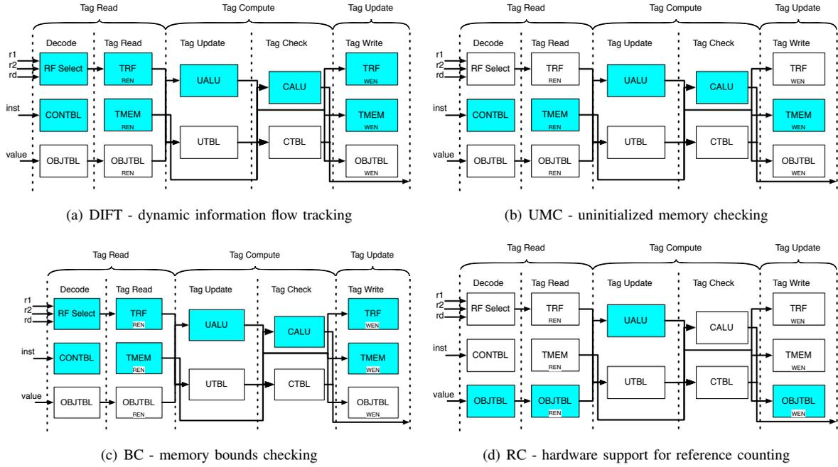
Fig. 5. Run-time monitoring techniques mapped to the Harmoni co-processor.
