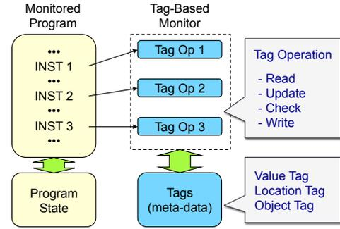
Fig. 2. Parallel run-time monitoring with tags.
