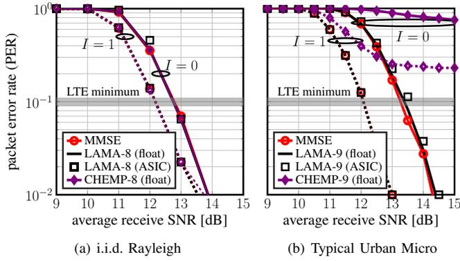
Fig. 5.  $256 \times 32$  massive MU-MIMO;  $R = 0.5$ ; 256-QAM; 9600 bits/packet.
