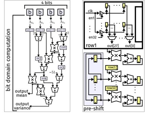
Fig. 4. Fan-out reduction of matrix-vector multiplication using Cannon's algorithm [10].
