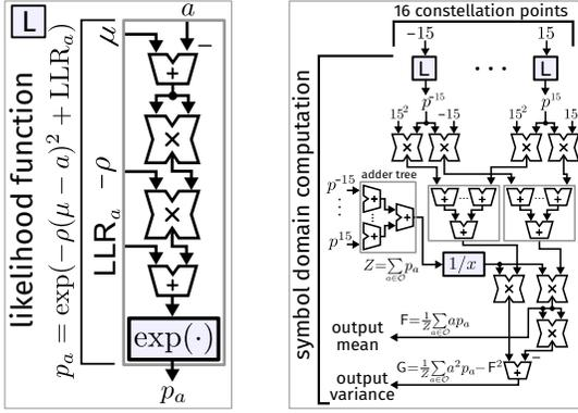
Fig. 2. Original MV unit for 256-QAM with separation into two 16-PAM units. Exact mean and variance computation entails high complexity and requires high arithmetic precision.
