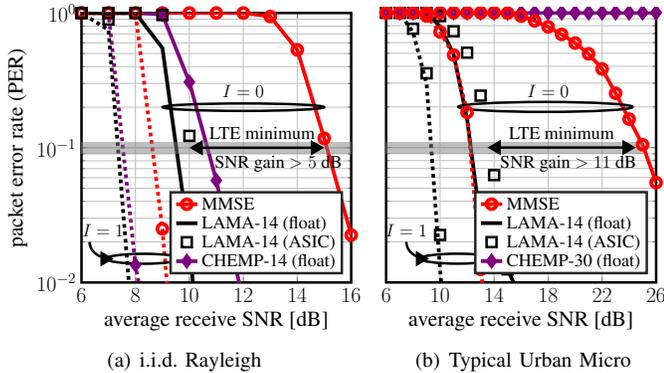
Fig. 6.  $32 \times 32$  massive MU-MIMO;  $R = 0.75$ ; QPSK; 3600 bits/packet.
