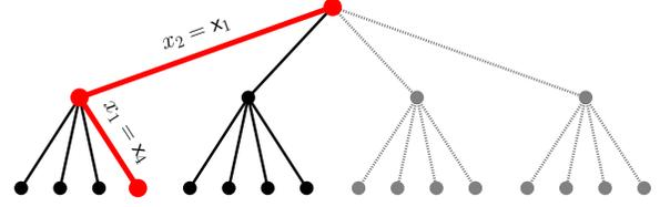
**Fig. 1:** Quaternary tree for the 1-bit-quantized case and for  $B = 2$ . Note that the root of the tree corresponds to the last entry of the vector  $\mathbf{x}$ , and that half of the tree can be pruned by symmetry (see Section 4.5). The path highlighted in red corresponds to the precoded vector  $\mathbf{x} = [x_4, x_1]^T$ .
