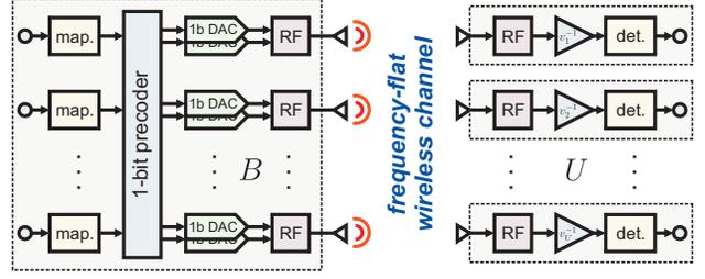
Fig. 1. Tx- and Rx-chains in the considered 1-bit precoded system.
