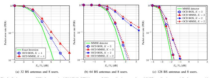
Fig. 2. Packet error rate (PER) for a massive MU-MIMO-OFDM system. BOX equalization outperforms MMSE equalization, especially for systems with a smaller BS-to-user antenna ratio. Furthermore, both approximate equalization methods achieve near-exact MMSE performance for a small number of iterations.
