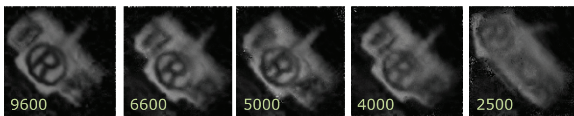
Figure 20. Performance for varying speed. We slowed down the operating speed of the SPC to indirectly increase object speed. The operating speed of the SPC is overlaid on top of the recovered video. Shown is a single frame from each recovered video, the instant corresponding to the pendulum swinging at maximum speed.
