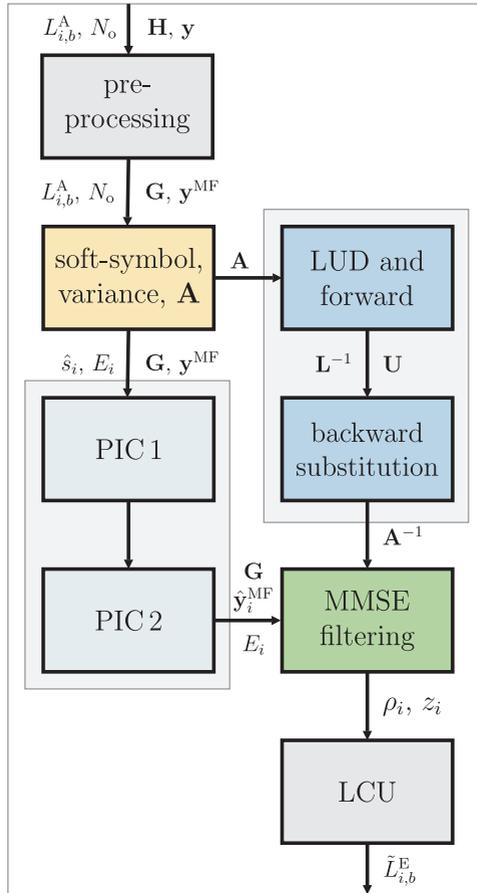
Figure 3.6: VLSI architecture of the SISO MMSE PIC detector.
