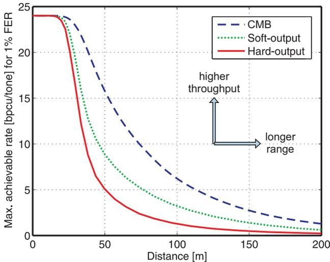
Figure 1.1: Distance (between transmitter and receiver) versus maximum achievable rates for 64-QAM data transmission in a 4-stream MIMO-OFDM system.
