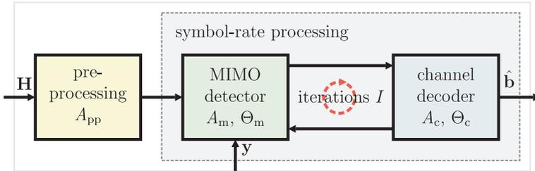
Figure 6.1: Iterative MIMO decoder with area and throughput figures.
