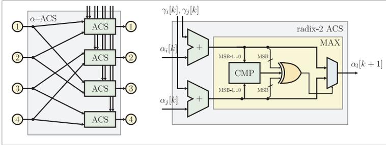
Figure 5.4: Left: architecture of a 4-state radix-2  $\alpha$ -ACS unit. Right: architecture of a radix-2 ACS unit with modulo normalization [36].
