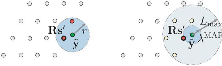
Figure 4.2: Left: the sphere constraint bounds the search to lattice points that are within a radius  $r$  around the received vector  $\tilde{\mathbf{y}}$  (the transmitted symbol vector is denoted by  $\mathbf{s}'$ ). Right: Extrinsic LLR clipping bounds the search for the MAP solution and all counter-hypotheses to  $r_{\max} = \sqrt{\lambda^{\text{MAP}} + L_{\max}}$ .
