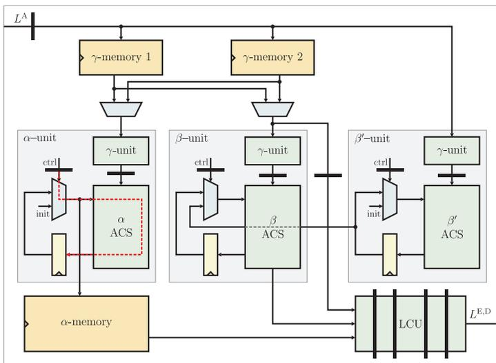
Figure 5.3: Overview of the M-BCJR architecture (the critical path in the ACS is highlighted).
