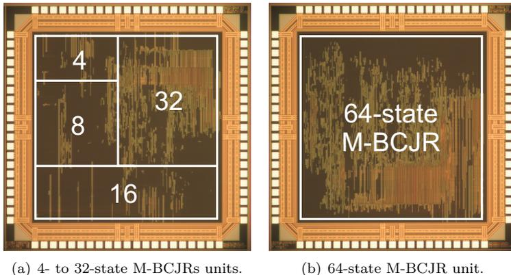
Figure 5.6: ASIC micrographs of high-throughput radix-2 max-log M-BCJR decoders in 180 nm (1P/6M) CMOS technology.
