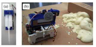
Fig. 5. (a) Bottom view of syringe dispenser for casting foam. The two compartments are actuated by the same plunger and both feed into a single static mixing nozzle. (b) Dispenser mounted on a small remote controlled robot. Cured previous depositions are shown right.
