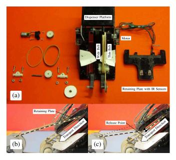
Fig. 4. Transport mechanism. (a) Top view of partially assembled mechanism. (b) Side view without toothpick. The thin belt (dashed line) moves past the retaining plate. (c) Side view with toothpick. A toothpick (cross mark) is transported along the retaining plate. As it moves, the toothpick increasingly deforms the thin belt. At the end of the plate, the thin belt releases and snaps back to its original position (dotted line) propelling the toothpick away from the mechanism.
