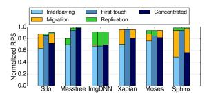
Fig. 3: Max load under various static (blue bars) and dynamic (yellow and green bars) data placement policies, normalized to an ideal policy with all local memory accesses (Arch 8 in Table III). Each application uses cores from 2 PIM stacks.
