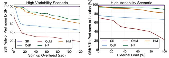
Figure 14: Sensitivity to spin-up time and external load.
