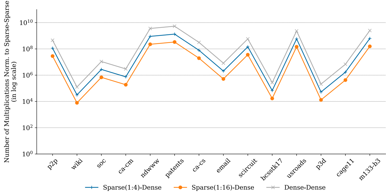
Figure 5.28: Normalized Number of Multiplications Performed in Different Sparsity Compression Levels – All numbers are normalized to the number of multiplications needed when representing both input matrices in a sparse format. In dense-dense, both matrices are stored in a dense format. In sparse(1:4)-dense and sparse(1:16)-dense, one matrix is stored in a sparse format with certain compression levels (i.e., one non-zero in a block of four or 16 contiguous elements), and the other is stored in a dense format.
