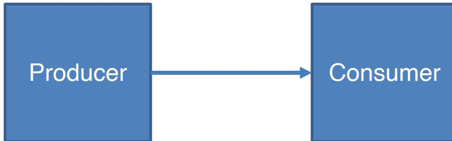
Communication channel that does not depend on the latency of the producer or the consumer
