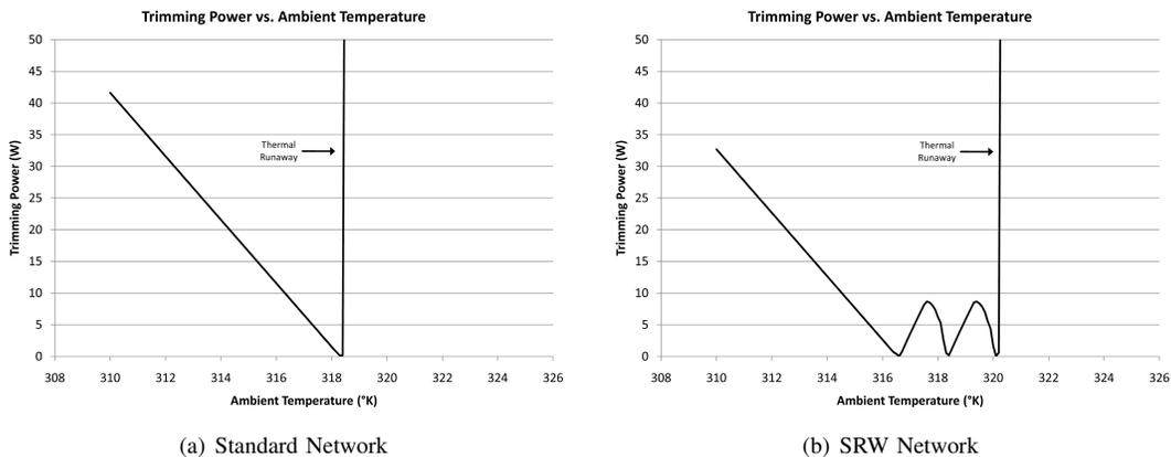
Fig. 1: Trimming Power (W) vs. Ambient Temperature ( $^{\circ}\text{K}$ ) for Standard Network (a) and Network Using SRW (b)
