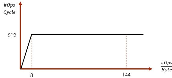
Figure 4: Roofline model for a convolution layer with  $stride = 1, 32 \times 3 \times 3$  filters, assuming we are using 256 DSPs, and that the DRAM bandwidth is 512 bits per cycle.
