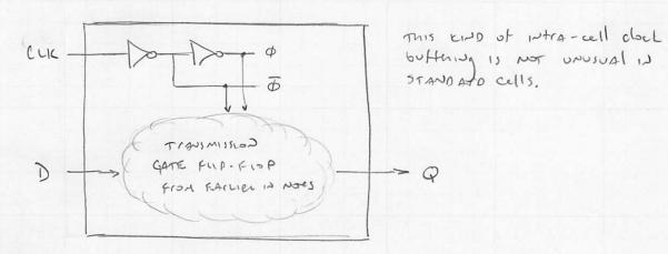
HOW Does mis impact me semp time, propagation delay, and most time? remember that all time of these metrics are retired with respect to the cik his of the cell not the local of and \$\overline{\pi}\$ signals
