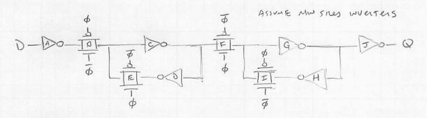
WE WANT TO CHAPACTERIZE THE SEND TIME, CLOCK-10-Q PROPAGATION DELAY AND THE MOS TIME
