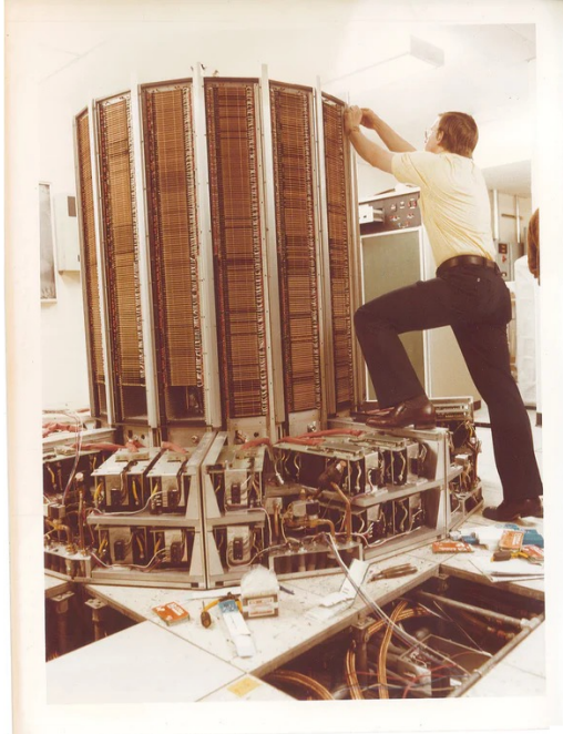
Cray 1 Supercomputer (1975) 160 Mega FLOPS 115 kW $7.9M ($40M today)
