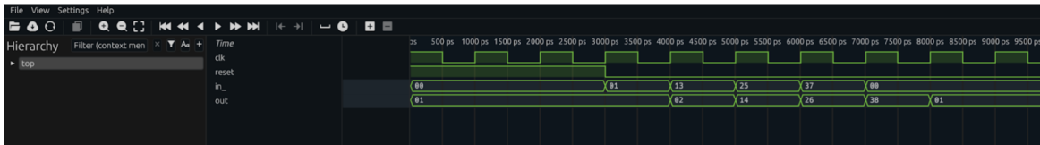
Figure 23: Surfer Waveform Viewer – Surfer is being used to browse the signals associated with the registered incrementer shown in Figure 16 and the ad-hoc test shown in Figure 24.
