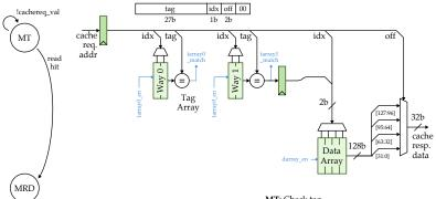
MT: Check tag MRD: Read data array, return cacheresp
