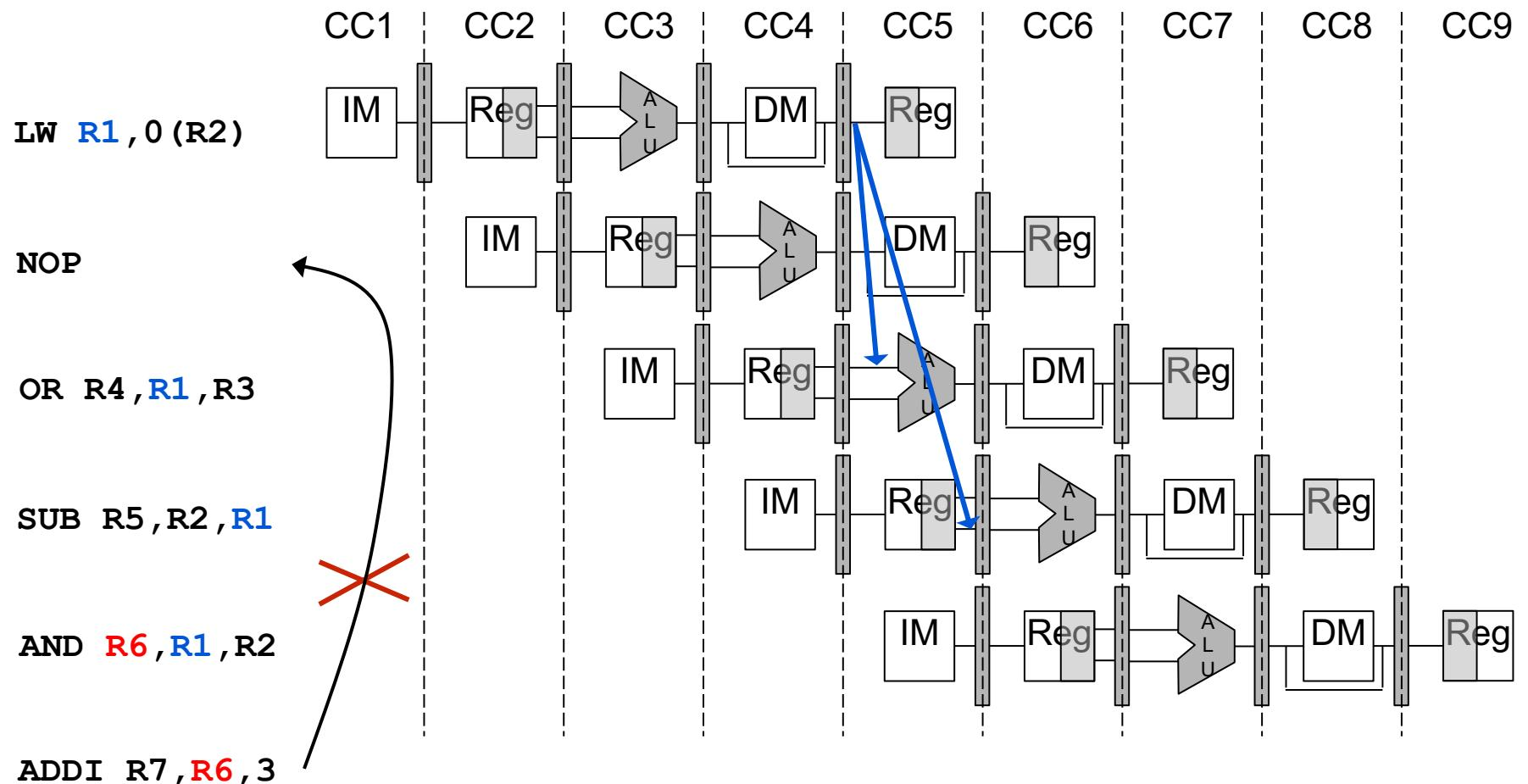
The ADDI instruction cannot be moved to the delay slot due to *data dependence on AND*
