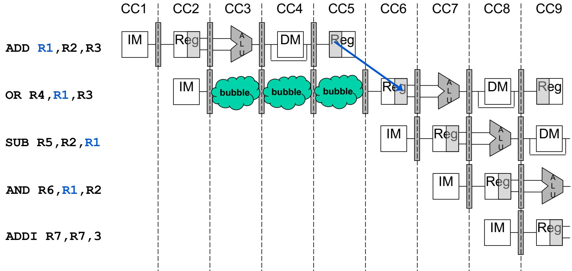
**Bubbles are inserted by HW to stall the pipeline for three cycles<sup>1</sup>**
