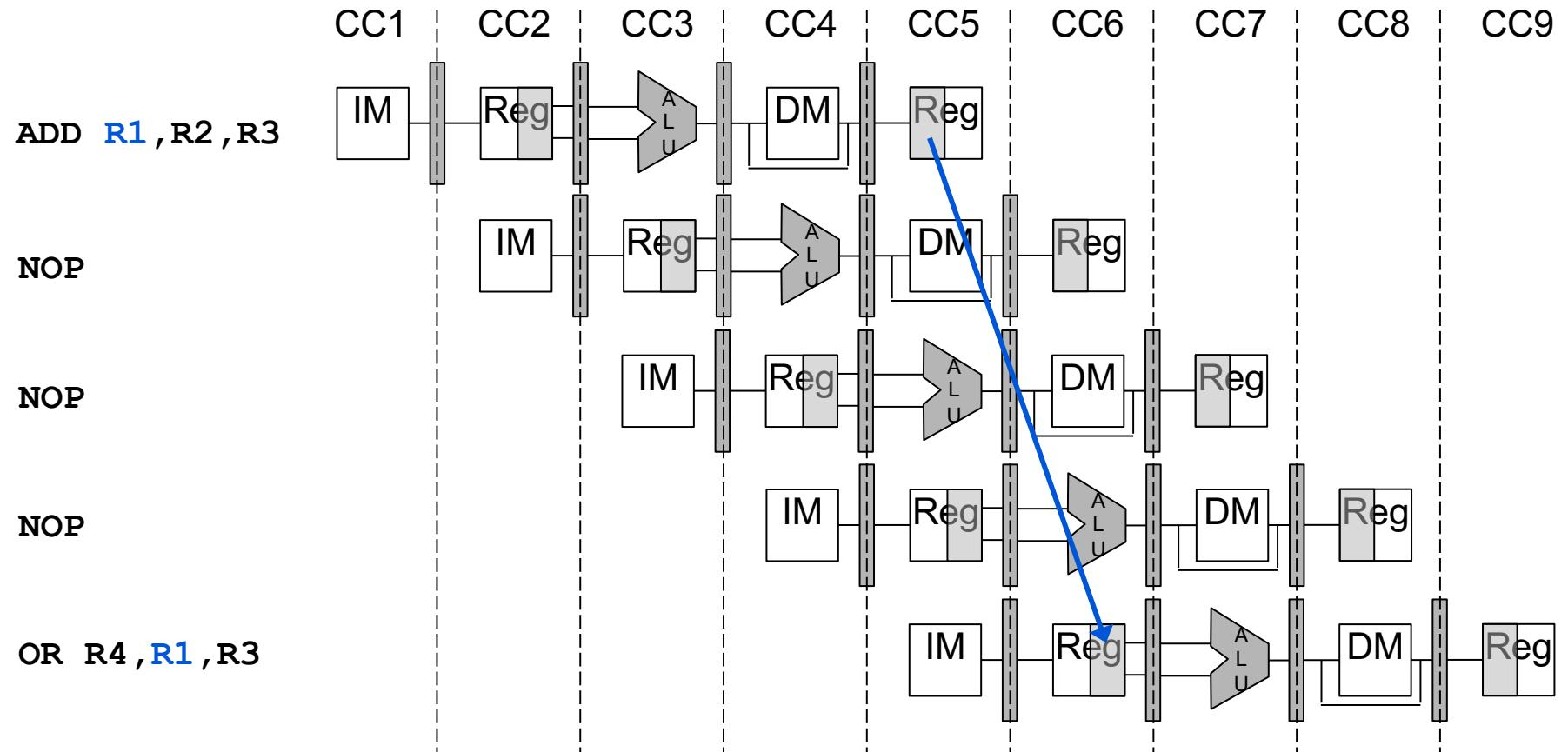
**NOP (No Operation)** does nothing when executed, which is commonly used as a dummy padding instruction to delay execution in a programs.
