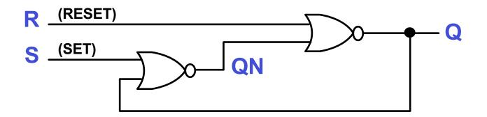
Suppose the S-R latch is initialized with Q=0, write down the next state given the following input sequence
