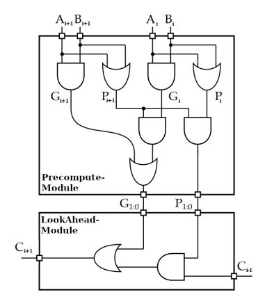
Fill in the table with the propagation and contamination delay of every path through the system containing both the precompute and look-ahead module (utilizing the previously stated timing parameters).
