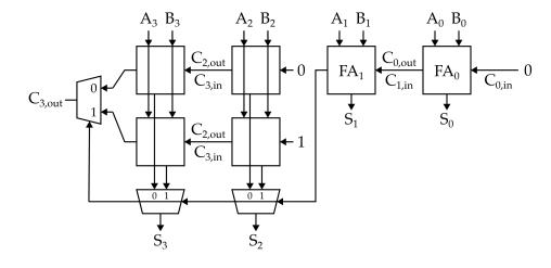
Compute the area of the four-bit carry-select adder in area units  $\alpha$  (without optimizing the full adders with constant carry-in).
