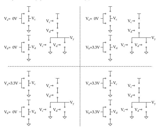
Complete the table. Mark closed transistors with C and open with 0.
