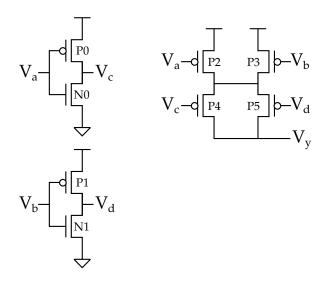
Check that all floating outputs and short-circuits were eliminated by filling out the table. Mark closed transistors with C.
