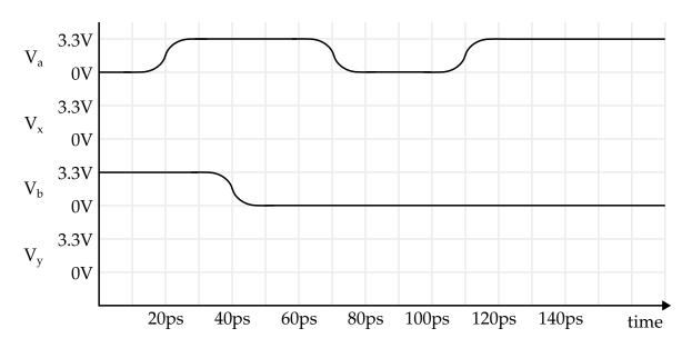
Part 4.C Timing Diagram with Constant Delay Model
