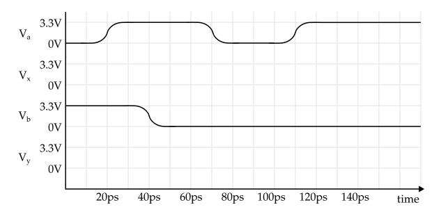
Part 4.E Timing Diagram with Transition- and Input-Dependent Constant Delay Model
