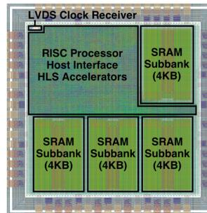
**Figure 1. BRGTC1 Test Chip** – A taped-out  $2 \times 2$  mm 1.3 M-transistor test chip in IBM 130 nm designed and implemented using our new PyMTL hardware modeling framework. Chip includes a simple pipelined 32-bit RISC processor, custom LVDS clock receiver, 16 KB of on-chip SRAM, and application-specific accelerators generated using commercial C-to-RTL high-level synthesis tools.
