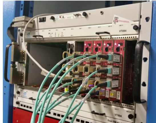
Figure 4. The demonstrator test system. The system is based on the CTP7 \mu TCA blade, used in the current CMS trigger. The system consists of four CTP7s. Each CTP7 has 63 input and 48 output 10 Gbps optical links.
