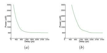
Fig. 1. Power-delay tradeoff curves for (a) a 16-bit adder and (b) a 16-bit multiplier.
