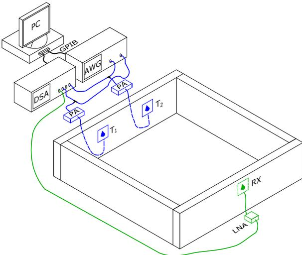
Fig. 4. Experimental setup to demonstrate spatial encryption.
