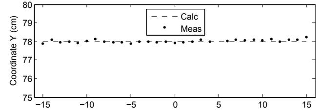
Fig. 18. Y-coordinate of the object during the sweep measurement.
