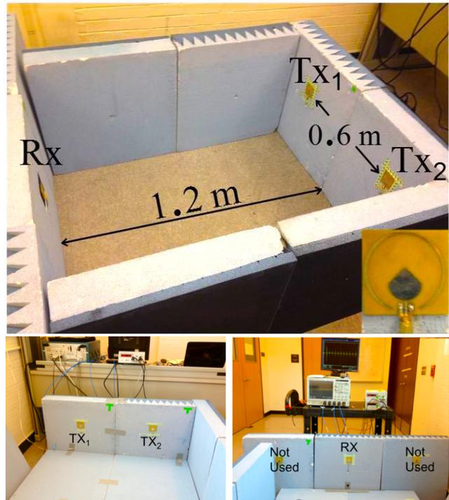
Fig. 8. Experimental setup to demonstrate spatial encryption (partially adapted from [2]).
