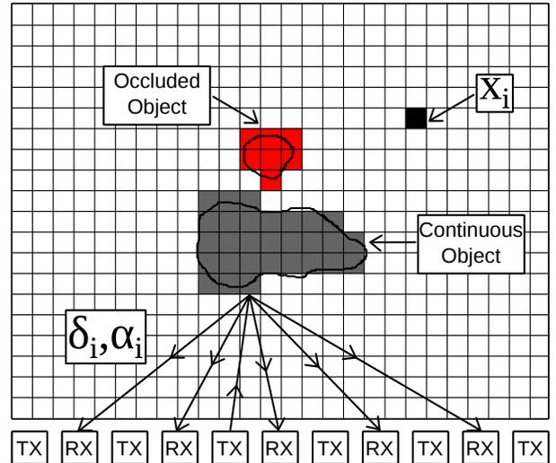
Fig. 20. Scene discretization and illustration of a scene where an object (red) is occluded by another object (grey). Scene recovery tries to identify the occupancy information contained in each cell  $x_i$  using the received signals.
