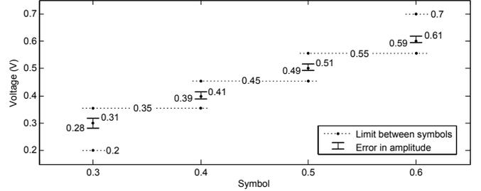
Fig. 5. Setting threshold midway between the symbol voltages (adapted from [2]).
