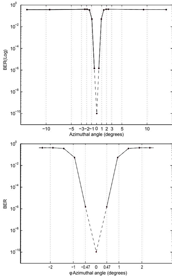
Fig. 7. Measured bit error rate (BER) of the system. (Top) Measurement across a wide range of azimuthal angle, (Bottom) Zoomed version between  $0-2^\circ$ . The BER measurement was done for the left side and mirrored the right side, leveraging symmetry in the system (adapted from [2]).
