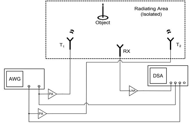
Fig. 11. Experimental setup for pulse-based time-of-flight localization
