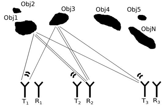
Fig. 19. Illustration of the proposed pulse-based time-of-flight imaging system consisting of  $M_T = 3$  transmitters and  $M_R = 3$  receivers. The goal is to recover scenes containing multiple complex objects.
