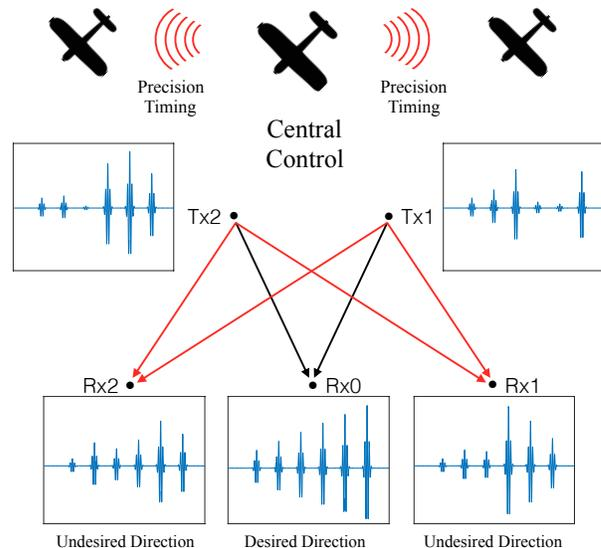
Fig. 9. Application of spatially secure point-to-point communication
