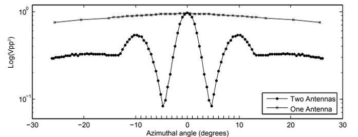
Fig. 6. Effective radiation patterns of a single antenna and two coherently transmitting antennas (adapted from [2]).
