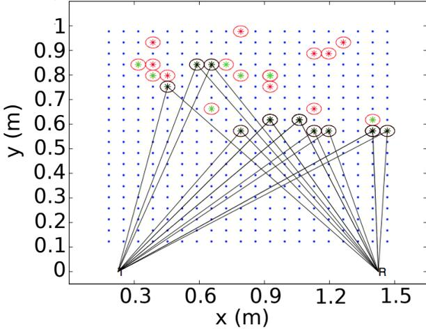
Fig. 21. Illustration of the ray-tracing method we used to synthesize the received signals in the presence of scenes with occlusions.
