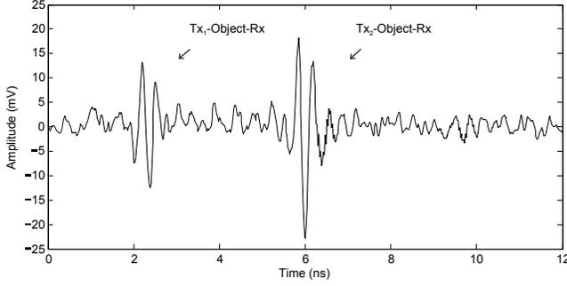
Fig. 15. Received signal after subtracting the background signature
