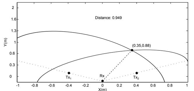
Fig. 13. Triangulation after receiving the signal
