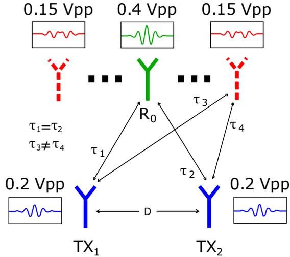
Fig. 2. Information generation with two tightly synchronized impulse transmitters. The correct information is only present at the desired location.
