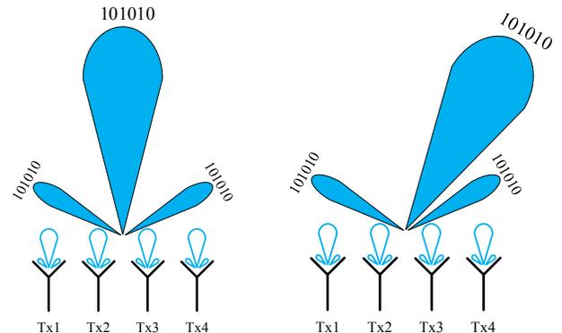
Fig. 1. Conventional beamforming of continuous wave (CW) based systems. The complete transmit information is present in the main lobe as well as in the side lobes. Any eavesdropper can receive and decode the information present in the side lobes.
