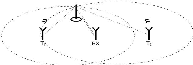
Fig. 10. Time-of-flight triangulation for localizing an object
