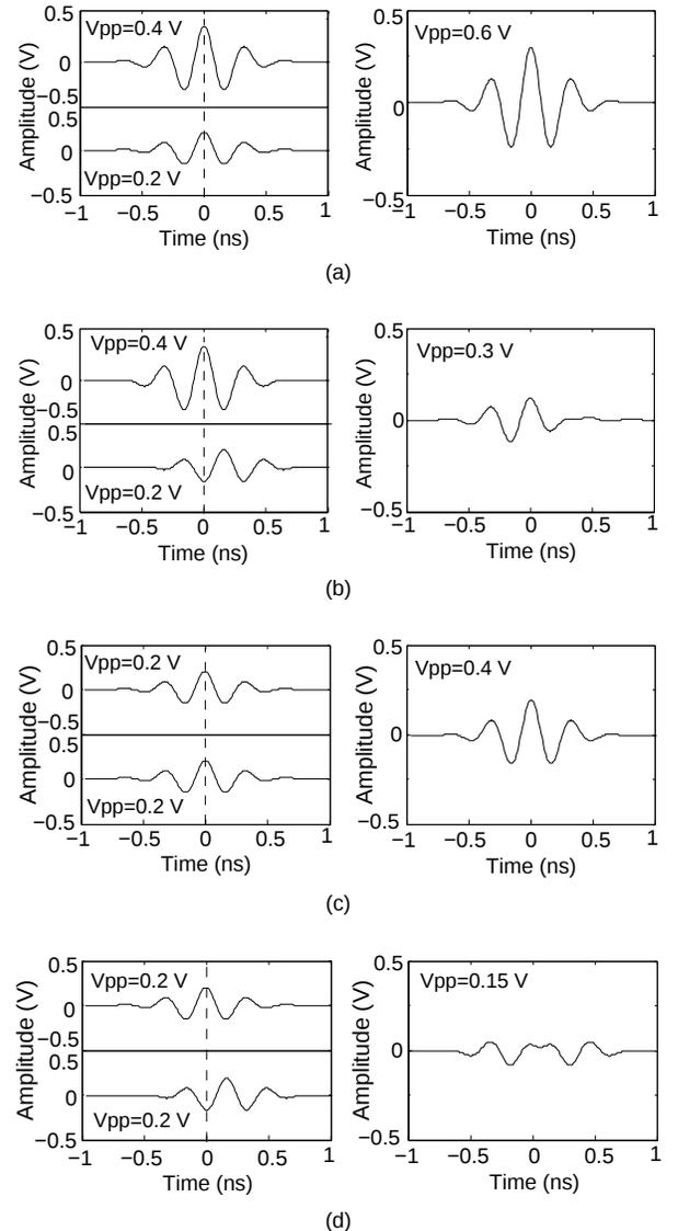
Fig. 3. The effect of time-delay in corrupting the time-domain waveforms. (Left) Time-domain signals generated by each antenna. (Right) The combined signal. (adapted from [2]).
