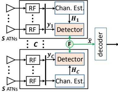
Fig. 1. Overview of the proposed decentralized data detection architecture.
