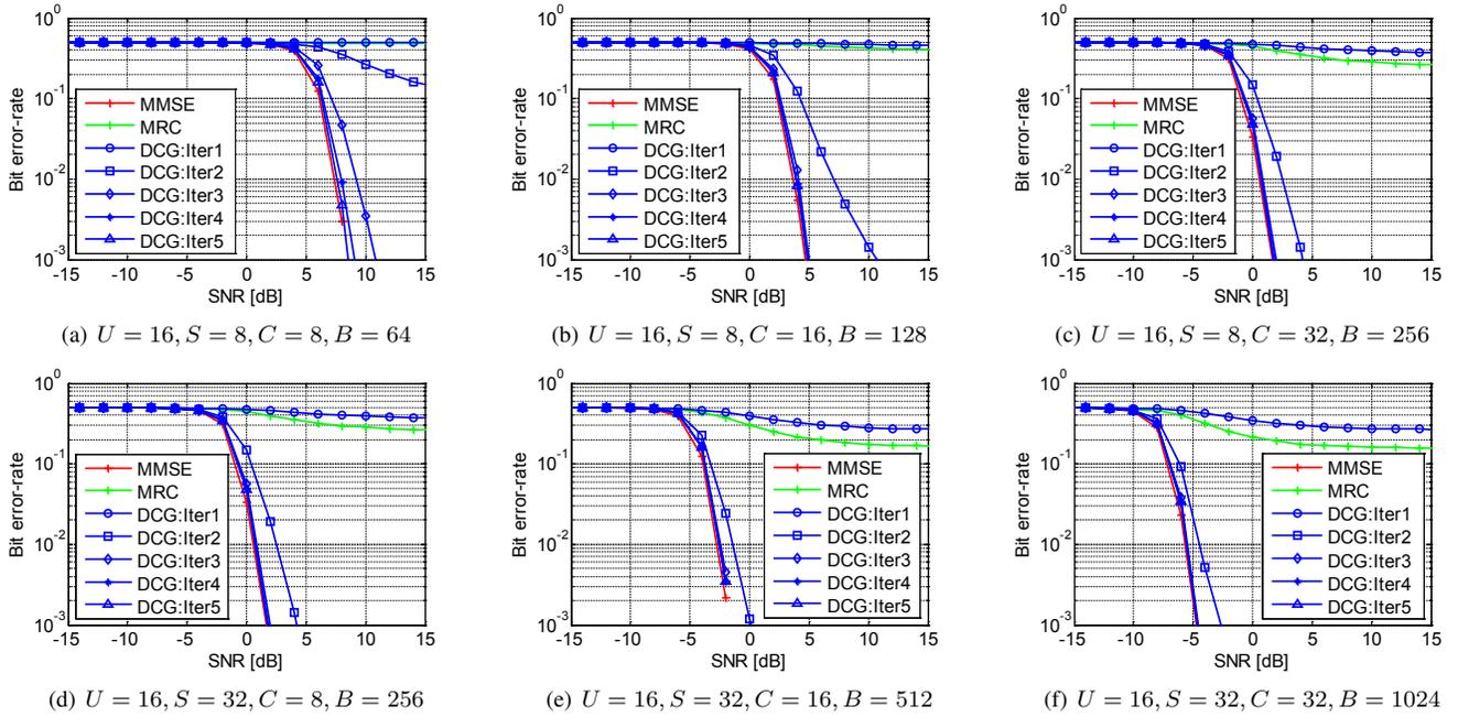
Fig. 2. Bit error rate (BER) performance comparison between decentralized conjugate gradient (DCG) and centralized MMSE detection for different system configurations:  $U$  denotes the number of users,  $S$  the number of antennas per cluster,  $C$  the number of antenna clusters, and  $B$  the number of BS antennas.
