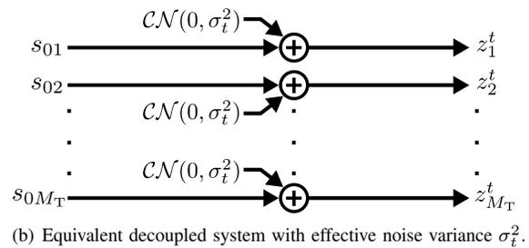
Fig. 1. IO-LAMA decouples large MIMO systems (a) into a set of parallel and independent AWGN channels with equal noise variance; (b) equivalent system in the large-system limit, i.e., for  $\beta = M_T/M_R$  with  $M_T \rightarrow \infty$ .
