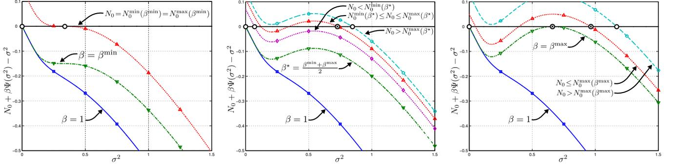
(a)  $\beta \leq \beta_{\mathcal{O}}^{\min}$ : IO-LAMA always converges to the unique, optimal fixed point (FP) irrespective of  $N_0$ . (b)  $\beta \in (\beta_{\mathcal{O}}^{\min}, \beta_{\mathcal{O}}^{\max})$ : IO-LAMA converges to the optimal FP if  $N_0 < N_0^{\min}(\beta)$  or  $N_0 > N_0^{\max}(\beta)$ . (c)  $\beta \geq \beta_{\mathcal{O}}^{\max}$ : IO-LAMA converges to the optimal fixed point if  $N_0 > N_0^{\max}(\beta)$ .
