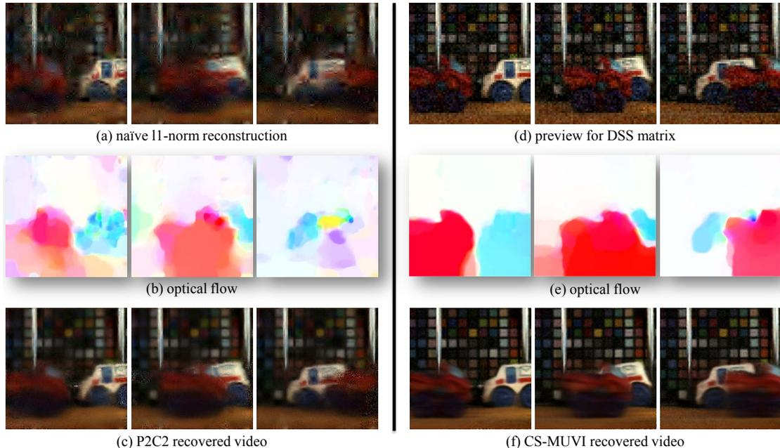
Figure 9. Comparison of the algorithm used for the P2C2 camera applied to SMC architectures with CS-MUVI recovery. Shown are frames of (a) naïve  $\ell_1$ -norm reconstruction, (b) the resulting optical-flow estimates, and (c) the P2C2 recovered video. The frames in (d) correspond to preview frames when using DSS matrices, (e) are the optical-flow estimates, and (f) is the scene recovered by CS-MUVI.
