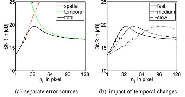
Figure 2. Trade-off between spatial and temporal approximation errors (measured in terms of the CS recovery SNR) for the scene in Fig. 1. (a) The SNRs caused by spatial and temporal approximation errors for different window lengths  $W$ . (b) The dependence of the total approximation error on the speed of the cross.
