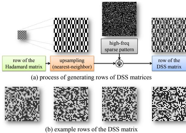
Figure 5. Generating DSS patterns. (a) Outline of the process in (7). (b) In practice, we permute the low-resolution Hadamard for better incoherence with the sparsifying wavelet basis. Fast generation of the DSS matrix requires us to impose additional structure on the high-frequency patterns. In particular, each sub-block of the high-frequency pattern is forced to be the same, which enables fast computation via convolutions.
