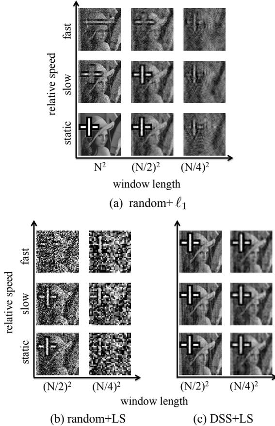
Figure 3. Comparison between (a)  $\ell_1$ -norm recovery, (b) LS recovery using a subsampled noiselet matrix, and (c) LS recovery using a dual-scale sensing (DSS) matrix of the scene in Fig. 1 for various relative speeds (of the cross) and window lengths  $W$ .
