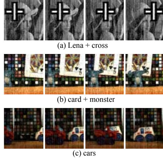
Figure 4. Preview frames for three different scenes. All previews consist of  $64 \times 64$  pixels. Preview frames are obtained simply using an inverse Hadamard transform, which opens up a variety of new (real-time) applications for video CS.
