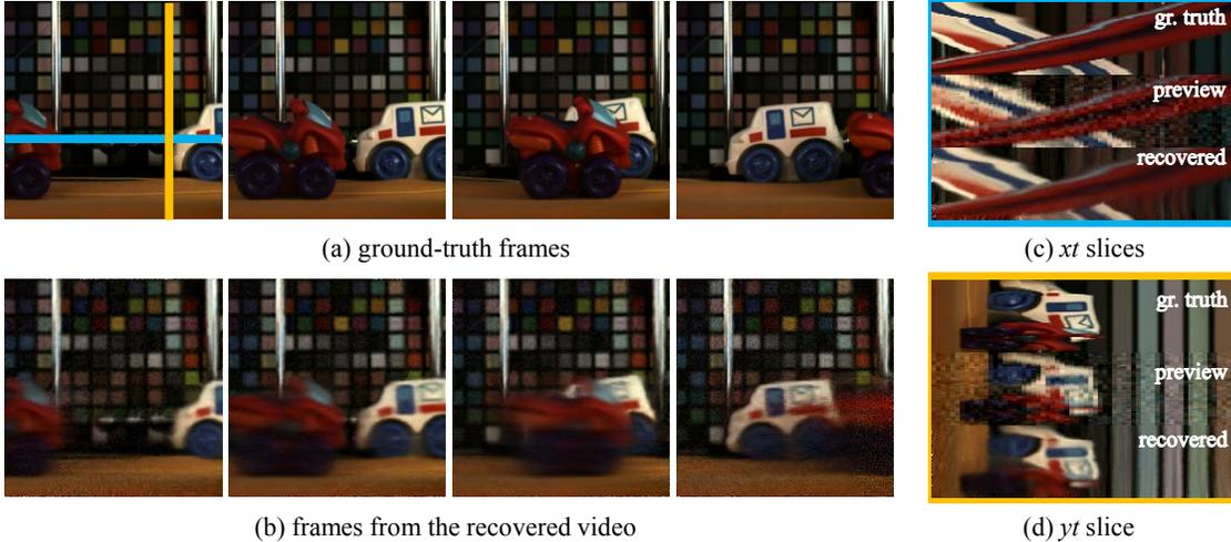
Figure 7. CS-MUVI recovery results of a video obtained from a high-speed camera. Shown are frames of (a) the ground truth and (b) the recovered video (PSNR = 25.0 dB). The  $xt$  and  $yt$  slices shown in (c) and (d) correspond to the color-coded lines of the first frame in (a). Preview frames for this video are shown in Fig. 4. (The  $xt$  and  $yt$  slices are rotated clockwise by 90 degrees.)
