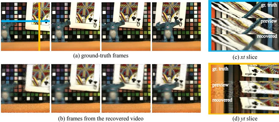
Figure 8. CS-MUVI recovery results of a video obtained from a high-speed camera. Shown are frames of (a) the ground truth and (b) the recovered video (PSNR = 20.4 dB). The  $xt$  and  $yt$  slices shown in (c) and (d) correspond to the color-coded lines of the first frame in (a). Preview frames for this video are shown in Fig. 4. (The  $xt$  and  $yt$  slices are rotated clockwise by 90 degrees.)
