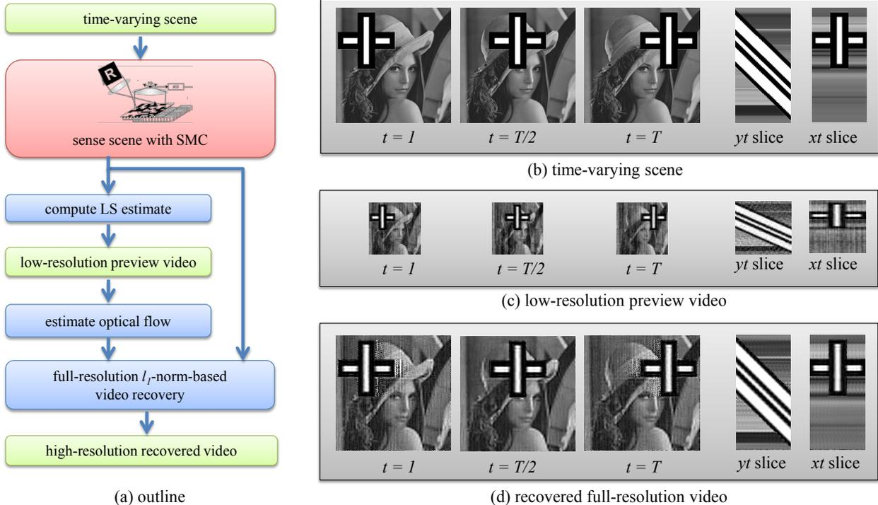
Figure 1. CS-MUVI example for a synthetic scene: (a) Flowchart of CS-MUVI, (b) ground-truth scene consisting of a background (Lena) and a single moving object (cross), (c) low-resolution preview video, and (d) high-resolution recovered video.
