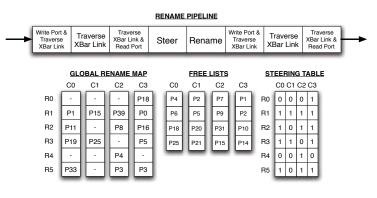
Figure 5: Rename pipeline (top) and illustrative example of SMU organization (bottom). R0 has a valid mapping in core three, whereas R1 has four valid mappings (one in each core). Only six architectural registers are shown.
