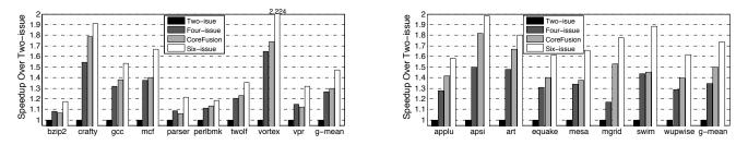
Figure 7: Speedup over FineGrain-2i when executing SPECINT (left) and SPECFP (right) benchmarks.
