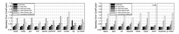
Figure 8: Speedups obtained when the FMU latency, rename pipeline depth, SMU dispatch bandwidth, operand crossbar delay, or the distributed ROB/LSQ are idealized.
