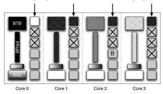
Figure 3: Example of aligned fetch in fused mode. In the figure, cores squash overfetched instructions as they receive a predict-taken notice from Core 2 with a two-cycle delay. The new target starts at Core 1, and thus Core 0 skips the first fetch cycle. Notice the banked branch predictor and BTB, the replicated GHR, and the Core-0-managed RAS.
