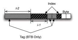
Figure 4: Configuration-oblivious indexing utilized in branch prediction and BTB. In the figure, i bits are used for indexing and t for tagging (tagging only meaningful in the BTB). Of course, i and t are generally not the same for branch predictor and BTB. Because of aligned fetch, the two tag bits sandwiched between index bits match the core number in the fused configuration.
