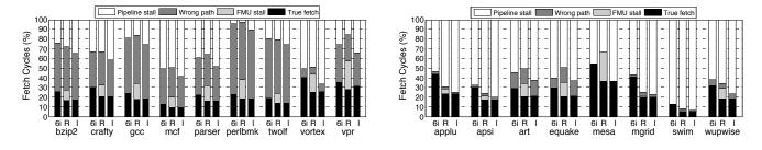
Figure 9: Distribution of fetch cycles on SPECINT (left) and SPECFP (right) benchmarks. 6i, R, and I denote our six-issue monolithic baseline, a realistic fused front-end with a two-cycle FMU delay, and an idealized fused front-end with no FMU delay, respectively.
