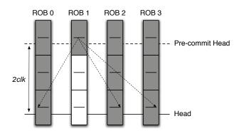
Figure 6: Simplified diagram of core fusion's distributed ROB. In the figure, ROB 1's head instruction pair is not ready to commit, which is communicated to the other ROBs. Pre-commit and conventional heads are spaced so that the message arrives just in time (2 clock cycles in the example). Upon completion of ROB 1's head instruction pair, a similar message is propagated, again arriving just in time to retire all four head instruction pairs in sync.
