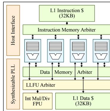
**Figure 1. Block Diagram of BRGTC2** – We paired the RISC-V ecosystem with productive open-source design tools to build a  $1 \times 1.25$  mm RISC-V system in TSMC 28 nm with seven graduate students in two months.
