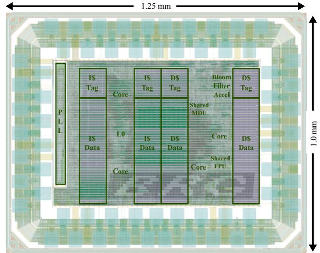
**Figure 2. Chip Plot of BRGTC2** – The research goal of the chip was to provide detailed performance, area, and energy numbers for various projects in our research group, while also evaluating the usability of synthesizable analog IP and experimenting with PyMTL support for ASICs.
