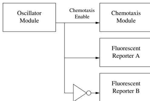
Figure 9: Schematic of Unsynchronized Chemotactic Oscillator
