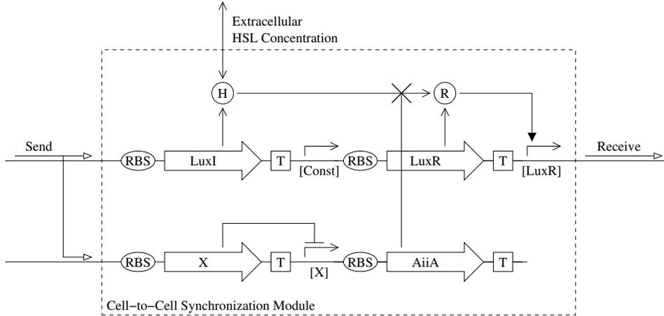
Figure 6: Schematic of Cell-to-Cell Synchronization Module with AiiA
