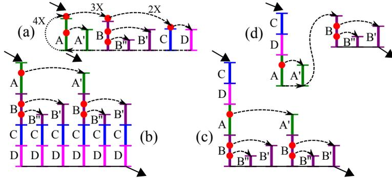
**Figure 3: Meta-Traces of One Simulated Cycle** – (a) event driven and static scheduling; (b) schedule unrolling; (c) heuristic topological sort; (d) trace breaking. A,B,C,D = traces of update blocks; red dots = guards that have bridges compiled from (connected by dashed arrows); A',B',B'' = conditional paths in update blocks that result in bridges; 4X,3X,2X = how many times the jump occurs in a simulated cycle; solid arrows = entry from and exit to the cycle loop.
