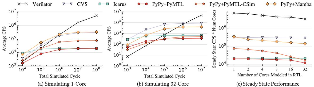
**Figure 4: Performance of Simulating RISC-V Multicore** – Each point in (a) and (b) is the average simulated cycle per second (CPS) taking compilation overhead into account; (c) captures the scalable performance: steady state CPS multiplied by number of simulated cores.
