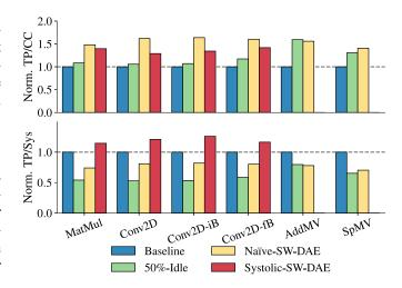
Fig. 7. Naïve and Systolic Software DAE: TP/CC = throughput per compute core; TP/Sys = overall throughput per system; MatMul showing  $768 \times 768$ ; Conv2D, Conv2D-iB, and Conv2D-fB showing 32 images batch; AddMV showing  $768 \times 768$ ; and SpMV showing FB-Johns55. See Table II for detailed input specification.
