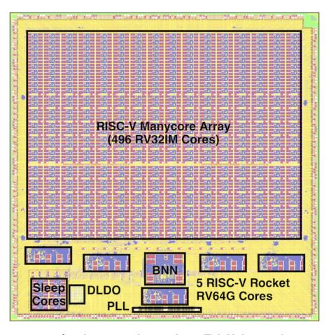
PyMTL2 played a small but important role in testing the BNN and automatically generating appropriate wrappers to interface with the Rocket core via RoCC
