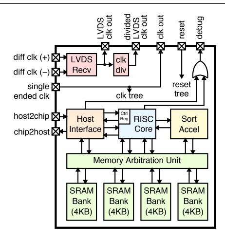
RISC processor, 16KB SRAM, HLS-generated accelerator 2x2mm, 1.2M-trans, IBM 130nm 95% done using PyMTL2
