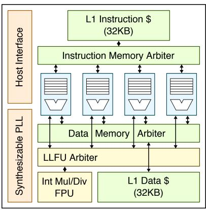
Four RISC-V RV32IMAF cores with "smart" sharing of L1\$/LLFU 1x1.2mm, 6.7M-trans, TSMC 28nm 95% done using PyMTL2
