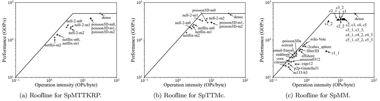
Figure 7: **Roofline evaluation of SpMTTKRP, SpTTMc and SpMM on Tensaurus** – the x-axis shows operation intensity which is number of operations (multiply and add) performed for each byte of data accessed from the off-chip memory; the y-axis shows the performance in GOP/s.
