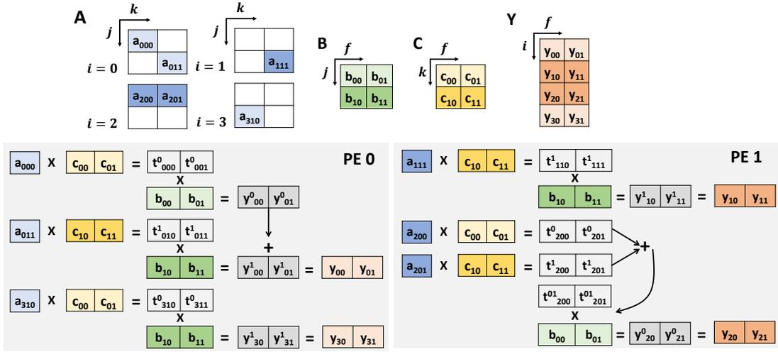
Figure 4: Execution of SpMTTKRP on two PEs.
