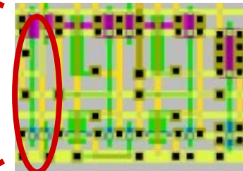
Standard Cell 2-16 gates per cell
