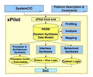
Fig. 1. xPilot system-level synthesis framework.
