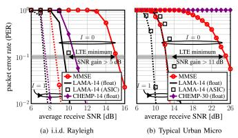
Fig. 6.  $32 \times 32$  massive MU-MIMO; R = 0.75; QPSK; 3600 bits/packet.
