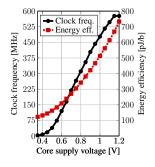
Fig. 8. Measured frequency and energy for different core voltages.
