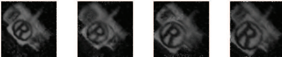
FIG. 21. Performance for varying size of dynamic object. For a wide range of object size, ranging from a quarter to half of the entire field-of-view of the camera, we obtain stable reconstructions.
