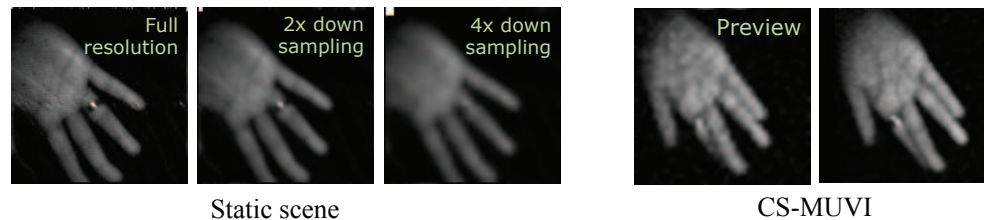
FIG. 18. Achieved resolution. We compare the achieved spatial resolution of the recovered video for a static target. For visual comparison, we artificially downsample the static image. It is clear that CS-MUVI recovers spatial resolution higher than a 2\times downsampling but slightly worse than the full resolution image.
