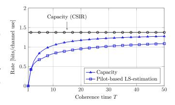
Fig. 2. Comparison of capacity (6) and the pilot-based LS-estimation lower bound (12) for the SISO case when  $\rho = 10$  dB.
