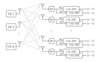
Fig. 1. One-bit massive MIMO uplink system model.
