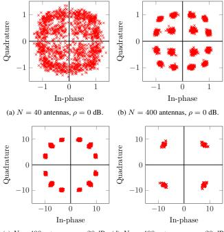
(c) N = 400 antennas,  $\rho = 20$  dB. (d) N = 400 antennas,  $\rho = 20$  dB, fully correlated channel coefficients.
