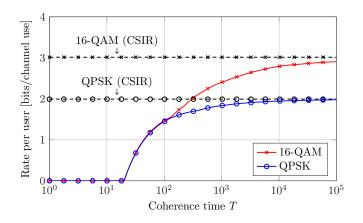
Fig. 5. Per-user achievable rate with LS estimation and MRC per user as a function of T; N = 400,  $\rho = -10$  dB, K = 20; the number of pilots P is optimized for each value of T.
