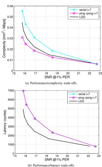
Fig. 8. Trade-off comparison of conventional serial and ping-pong architectures to LDD using 16-QAM.
