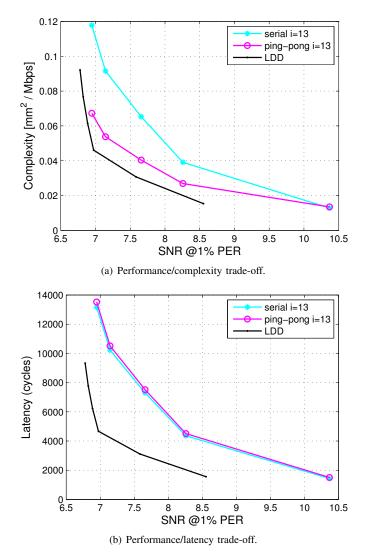
Fig. 7. Trade-off comparison of conventional serial and ping-pong architectures to LDD using QPSK modulation.
