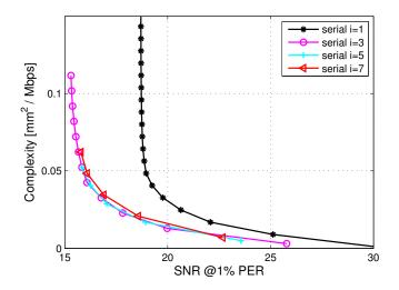
Fig. 5. Performance/complexity trade-off of the serial IDD schedule. Each simulation point corresponds to the number of outer iterations I, whereas each curve is associated to a different number of inner iterations i. (Simulated for a 1296 bit codeword with 16-QAM.)
