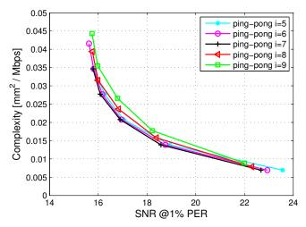
Fig. 6. Performance/complexity trade-off of the ping-pong IDD schedule. Each simulation point corresponds to the number of outer iterations I, whereas each curve is associated to a different number of inner iterations i. (Simulated for a 1296 bit codeword with 16-QAM)
