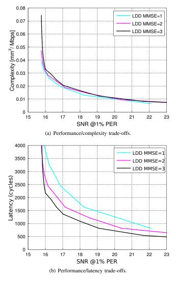
Fig. 9. LDD complexity and latency with different ratios between MMSE-PIC and LDPC operations for 16-QAM.
