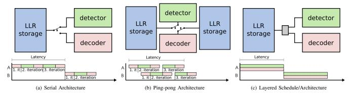
Fig. 2. High-level architecture overview and corresponding time diagrams for the three considered iterative MIMO-receiver architectures.
