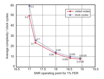
Figure 4.20: Average complexity of the soft-output STS-SD algorithm compared with the average number of clock cycles of the corresponding VLSI implementation (with MMSE-SQRD preprocessing). The numbers next to the curves correspond to normalized LLR clipping levels.
