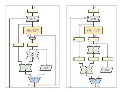
Figure 3.8: Two architectures for computation or reciprocals. Left: iterative architecture; right: pipelined architecture.
