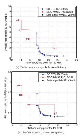
Figure 6.6: Tradeoffs: SISO MMSE PIC, SO STS-SD, and linear softoutput MMSE detection for convolutional codes.
