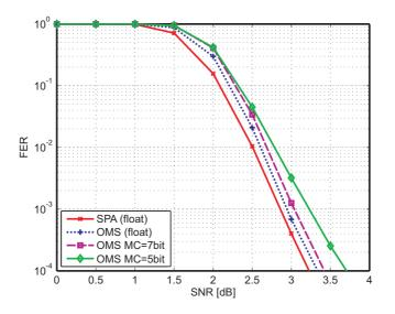
Figure 5.10: Frame error rate (FER) comparison using the R = 1/2, Z = 81 code [2] in an AWGN channel using BPSK modulation.
