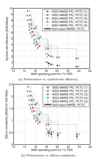
Figure 6.4: Performance/complexity trade-offs for SISO MMSE PIC and linear soft-output MMSE detection (both using PCTCs.)
