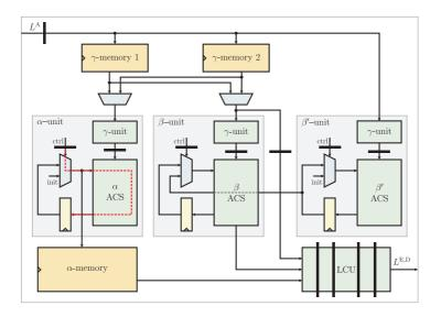
Figure 5.3: Overview of the M-BCJR architecture (the critical path in the ACS is highlighted).
