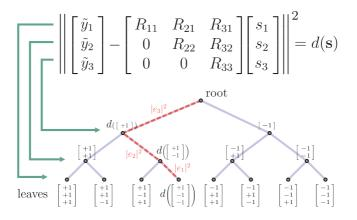
Figure 4.1: Example of the weighted tree for a MIMO system with  $M_{\rm T}=3$  and BPSK modulation.
