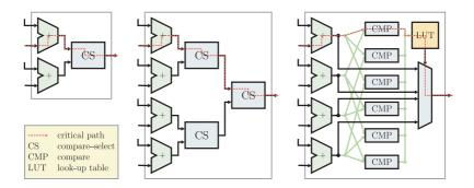
Figure 5.16: Left: radix-2 ACS. Middle: slow radix-4 ACS. Right: fast radix-4 ACS. The critical paths are indicated with dashed lines.
