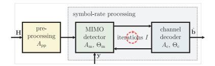
Figure 6.1: Iterative MIMO decoder with area and throughput figures.
