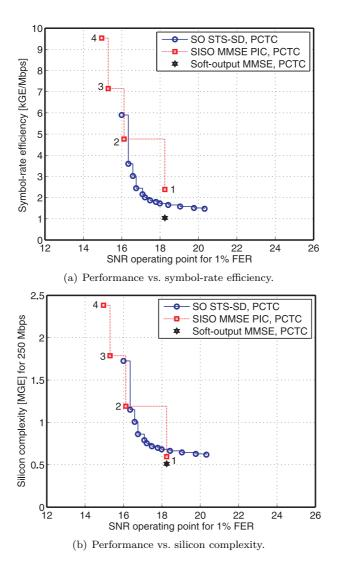
Figure 6.8: Tradeoffs: SISO MMSE PIC, SO STS-SD, and linear soft-output MMSE detection for turbo codes.
