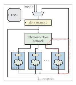
Figure 3.7: Architectural principle underlying each PU.
