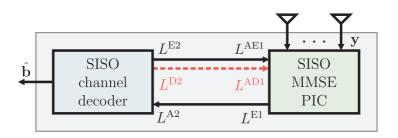
Figure 3.1: Iterative MIMO decoder using the SISO MMSE PIC detector and a channel decoder that provides extrinsic  $L^{E2}$  and intrinsic  $L^{D2}$  (corresponding to the dashed line) a posteriori LLRs [43].
