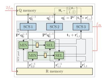
Figure 5.8: Architectural details and decoding schedule of the QC-LDPC decoder for Z = 2 and  $N_b = M_b = 2$ .
