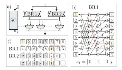
Figure 5.9: Subset cyclic shifter architecture: a) overview, b) barrel rotator, and c) operation principle for  $Z_{\text{max}} = 8$ , Z = 6, and c = 1.
