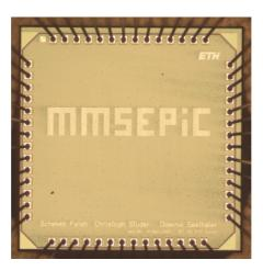
Figure 3.10: ASIC micrograph of the SISO MMSE PIC detector in 90 nm (1P/9M) CMOS technology.
