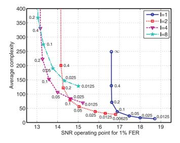
Figure 4.8: Performance/complexity tradeoff of SISO STS-SD with SQRD. The numbers next to the curves correspond to normalized LLR clipping parameters.
