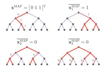
Figure 4.4: Example of the prepruning procedure (BPSK constellation,  $M_{\rm T} = 3$ ) of the RTS algorithm [125]. Counter-hypotheses to the MAP solution are found by forcing SD through the dashed branches.
