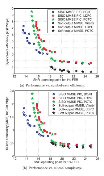
Figure 6.5: Tradeoff summary for SISO MMSE PIC and linear softoutput MMSE detection using different channel decoders.
