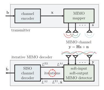
Figure 2.1: MIMO wireless communication system employing BICM, spatial multiplexing (SM), and iterative MIMO decoding [19].
