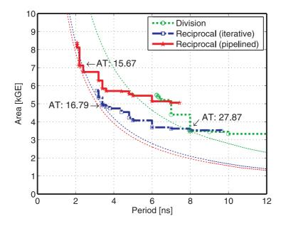
Figure 3.9: AT trade-off of division unit and two different reciprocal units in 130 nm (1P/8M) CMOS technology.
