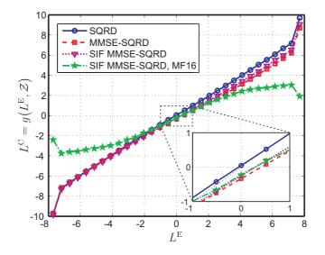
Figure 4.12: Different LLR correction functions for I = 1 at SNR = 16 dB using  $\mathcal{Z} = \{L_{\text{max}}, D_{\text{avg}}, SNR, T\}.$
