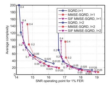
Figure 4.9: Performance/complexity tradeoff of SISO STS-SD with SQRD, MMSE-SQRD, and SIF MMSE-SQRD. The numbers next to the curves correspond to normalized LLR clipping parameters.
