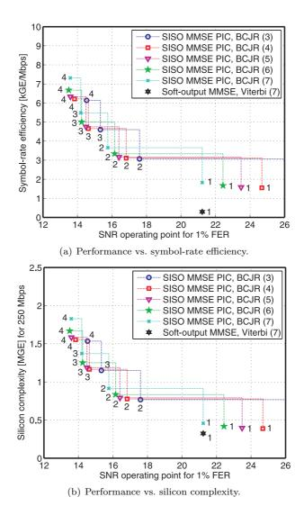
Figure 6.2: Performance/complexity tradeoffs for SISO MMSE PIC with M-BCJR decoding compared to linear soft-output MMSE detection with Viterbi decoding.
