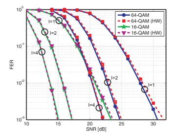
Figure 3.11: Fixed-point performance results for 64-QAM and 16-QAM of the SISO MMSE PIC implementation. Dashed lines correspond to the fixed-point hardware (HW) performance.
