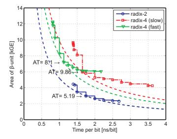
Figure 5.17: A rea-time tradeoff comparison of radix-2 and radix-4  $\beta$ unit ACS in 180 nm CMOS technology. The dashed lines represent constant area-time (AT)-product.
