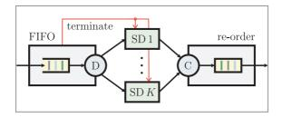
Figure 4.5: FIFO scheduling with K parallel SD-cores.
