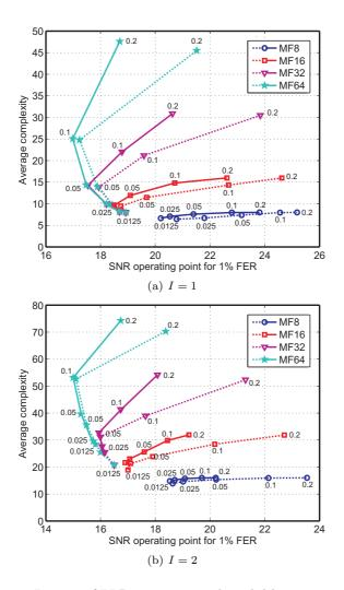
Figure 4.13: Impact of LLR correction. The solid lines correspond to the performance obtained with LLR correction, whereas the dotted lines pertain to un-corrected LLRs. Both variants employ early termination with MF scheduling and compensation of self-interference in the LLRs in combination with MMSE-SQRD.
