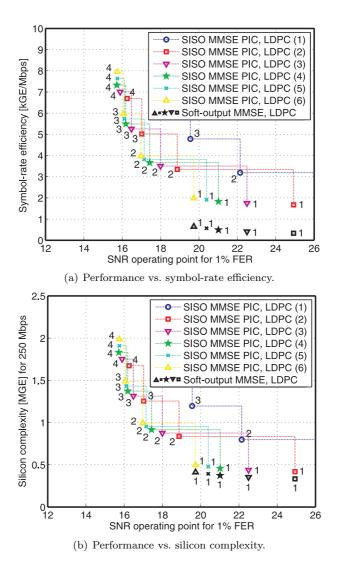
Figure 6.3: Performance/complexity tradeoffs for SISO MMSE PIC and linear soft-output MMSE detection (both with LDPC codes).
