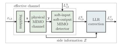
Figure 4.6: LLR correction post-processes the LLRs resulting from the effective channel using side information  $\mathcal{Z}$ .
