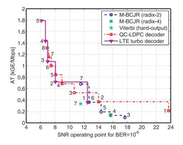
Figure 5.19: Hardware-based performance/complexity tradeoff for SISO channel decoders. The numbers next to the M-BCJR decoder corresponds to the constraint length. The numbers next to the QC-LDPC and LTE turbo decoder denote the number of iterations.
