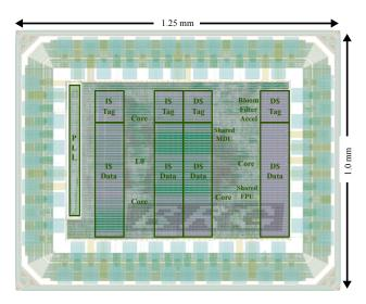
**Figure 2. Chip Plot of BRGTC2** – The research goal of the chip was to provide detailed performance, area, and energy numbers for various projects in our research group, while also evaluating the usability of synthesizable analog IP and experimenting with PyMTL support for ASICs.
