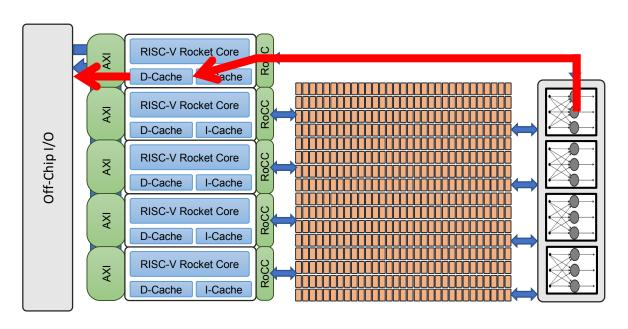
The BNN specialized accelerator can use one of the Rocket cores' caches to load every layer's weights; but, it is inefficient due to off-chip traffic
