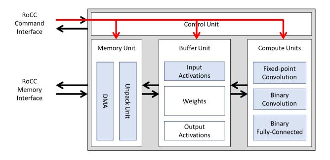
Accelerator is configured to process a layer through RoCC command messages
